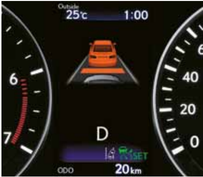
Multi-information display Positioned in the center of the meter cluster, the 4.2-inch colour Thin Film Transistor (TFT) multi-information display provides a wide range of vehicle information, data, and warnings.
