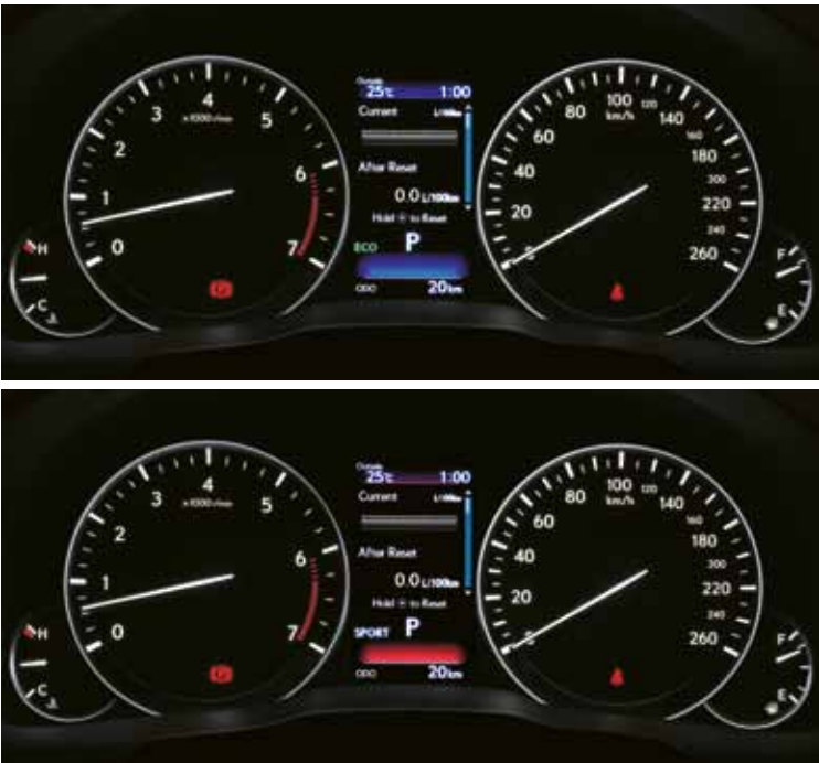
Optitron meters The easy-to-read Optitron meters provide critical driving information at a glance. An Eco Driving Indicator informs the driver when accelerator operation is considerate to the environment. In Eco and Normal Modes, the instrumentation turns a tranquil blue. Switching to Sport Mode illuminates the instrumentation in a vibrant red.
