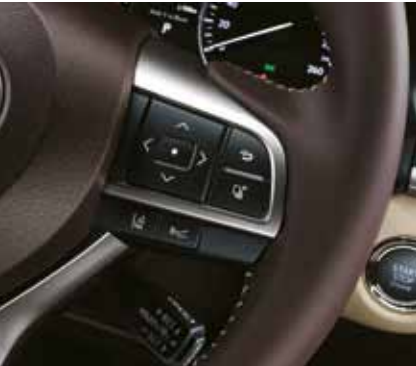
Steering wheel controls The ergonomically designed steering wheel has built-in switches so the driver can control a variety of vehicle systems, including the audio system and multi-information display, while keeping both hands on the steering wheel.
