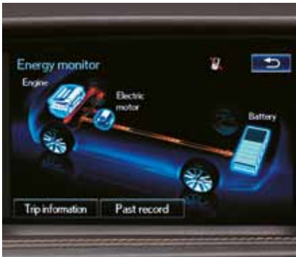
Regenerative braking The regenerative brake system activates the motor as a generator while decelerating and braking, converting the moving vehicle's kinetic energy into electric energy and using it to charge the battery.
