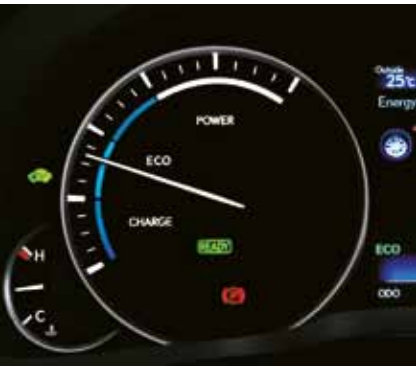
EV (Electric Vehicle)-Drive Mode EV-Drive Mode limits starting of the engine to enable the car to be driven using only motor power up to speeds of approximately 40km/h. It is designed to enhance quietness while driving in residential areas late at night, and to reduce emissions in indoor car parks and garages.*
