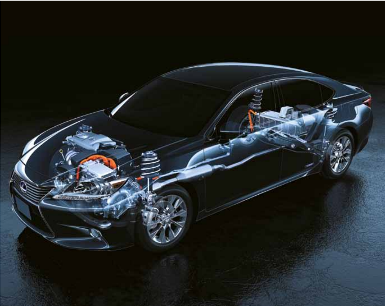
For dynamic driving and exceptional environmental performance, Lexus Hybrid Drive intelligently combines the power of a highly-efficient 2.5-litre petrol engine with electric power from a high-output motor.
