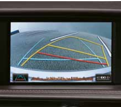
Parking Assist Monitor It supports smooth reversing operations when parking in a garage or parallel parking, showing the rear view taken by a camera integrated into the rear of the vehicle, together with guidelines on the EMV display.*3
