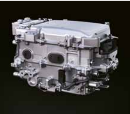
Power control unit The brain of the Lexus Hybrid Drive, the power control unit optimises control of DC electricity from the battery and AC electricity for driving the motor and generator. It also boosts battery voltage for extracting maximum power from the motor and generator.
